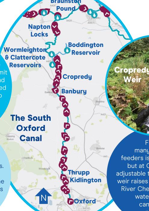
Flow in many of these feeders is uncontrolled, but at Cropredy an adjustable tilting steel river weir raises the level of the River Cherwell to divert water into the canal when needed
